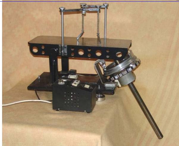
Figure 3.1 Tribometer based on angular measurements
